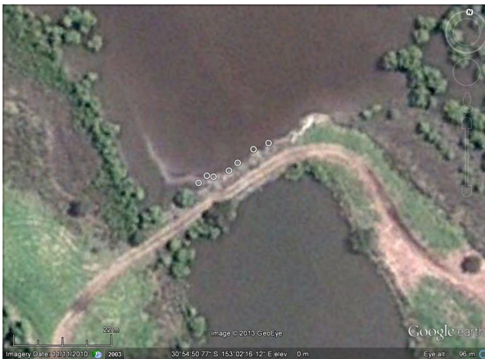
Figure 27 Location of points of discharge through berm into Juncus Inlet during low tide conditions
