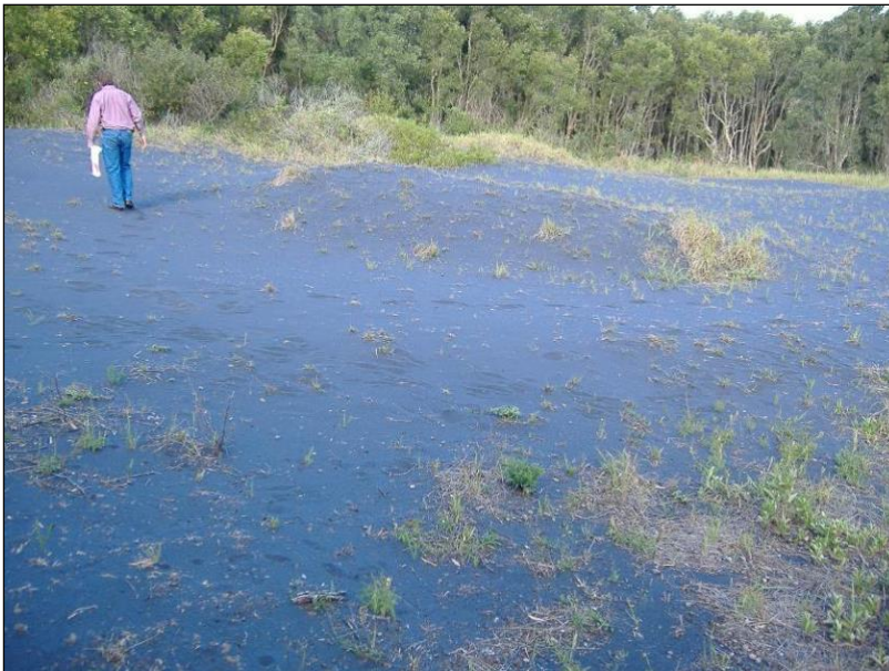
Figure 13. Abandoned Ilmenite tailings dump Noosa North Shore (photo taken in 2007) prior to removal by Green Coast Resources.
