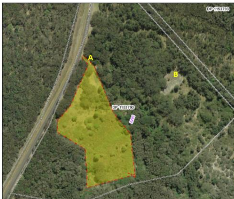
Figure 2. Aerial image of Lot 2281 DP1153793. Approximate outline of ilmenite stockpile/dump in yellow showing access from Point Plomer Road (A) and site of former MDL mineral separation plant site (B). Approximate surface area of ilmenite pile 2 Ha.
