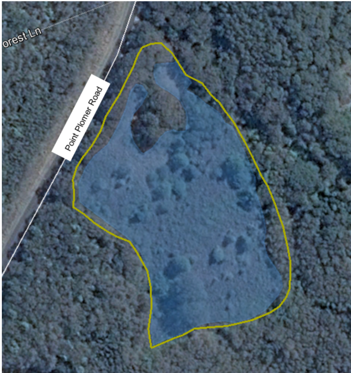
Figure 4 Approximate ilmenite stockpile boundary shown in yellow. Area to be grubbed and raked shown in blue. Remnant native vegetation outside the blue area shall be marked with flagging tape and remain undisturbed during relocation of the stockpile
