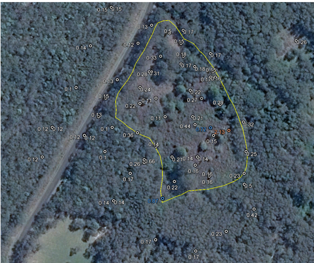
Figure 2. Detail view of Crescent Head ilmenite stockpile and background field gamma readings ( \mu\text{Sv}/\text{hour} ), with approximate stockpile outline shown in yellow.
