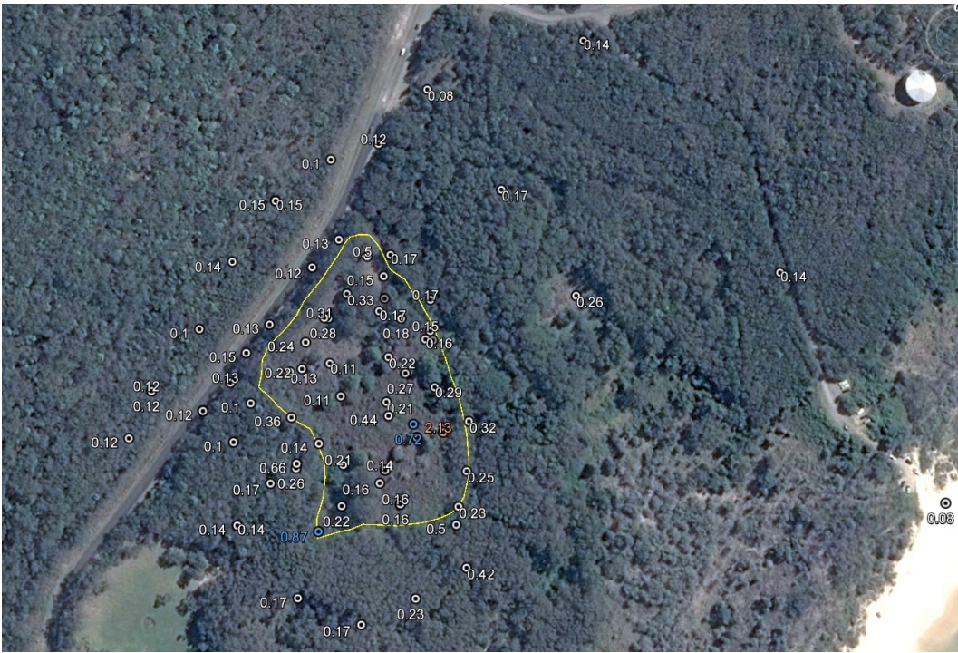
Figure 1. Overview of Crescent Head stockpile site and background field gamma readings ( \mu\text{Sv}/\text{hour} ), with approximate stockpile outline shown in yellow.
