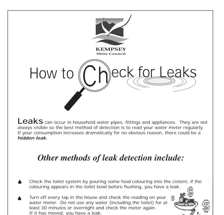
Some meters have a leak detection dial. If it is moving when there is no water being used, you have a leak.
